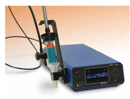
Positive displacement dispensers are ideal for applying uniform amounts of 2-part epoxies and other fluids that change viscosity over time. Compressed air is not required—instead, these electrically operated units use stepper motors and patented technology to advance and retract a piston inside the syringe barrel. They will produce accurate, repeatable deposits, regardless of changes in fluid viscosity or temperature.
